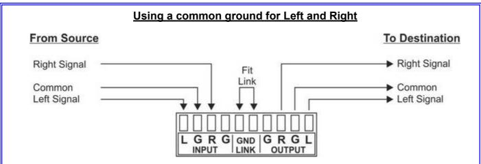
Always use screened cables for connection between the signal source and the LVC-51 as well as between the LVC-51 and the signal destination.
